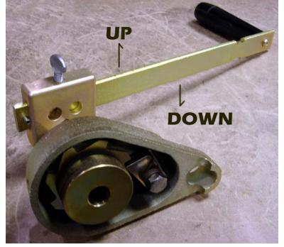
For proper use and long life, the Weston-style brakes require the wire rope to be wound onto the winch drum in only one direction. **Improper wire rope installation will prevent the brake from working properly and the load could fall.** Also, with this type of brake assembly, a free-spool option is typically not available.
