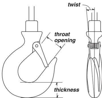
**The wire rope assembly must be replaced if the throat opening is 15% wider than nominal, if the thickness is 10% less than nominal, or if the hook is twisted 10° or more.**
