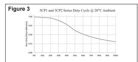
The duty cycle data shown in figure 2 was collected with a 20°C ambient temperature. Ambient temperatures above and below this will have an effect on the duty cycle.
